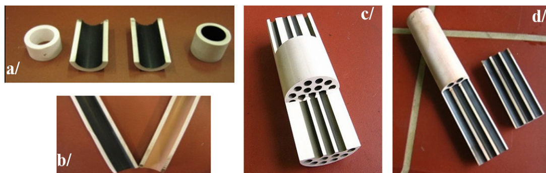
Fig. 2. Asymmetric tubular ceramic membranes coated with the impregnation/decomposition procedure of Pd acetate: (a) single channel \text{Al}_2\text{O}_3 membrane coated with Pd; (b) single channel \text{TiO}_2 membrane with bimetallic coating Pd/Au (left) and pure Au coating (right); (c) 19-channel \text{Al}_2\text{O}_3 membrane coated with Pd; (d) 7-channel \text{Al}_2\text{O}_3 membrane coated with Pd.
